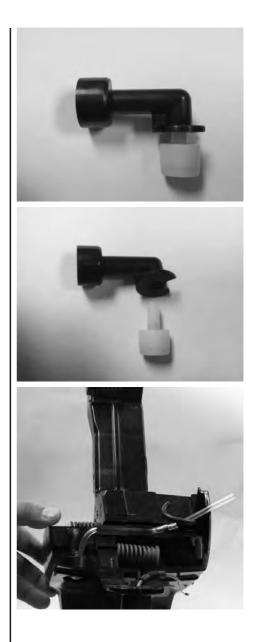
19.17 Shock Absorbers Using the Workshop Key Torx T27 (P/N 546191), remove shock absorbers.
