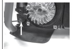
Separate fuel tank from crankcase by pulling up on the crankcase while holding the fuel tank.
