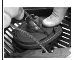
9.5 Pulley removal from spring.
