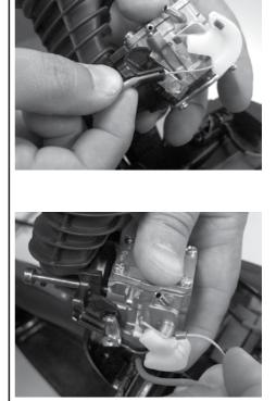
10.8 Remove clutchside flange screw (P/N 544072) and screw (P/N 544065).
