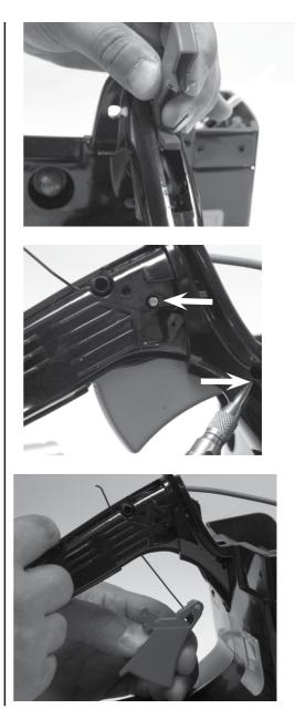
Remove throttle cable (P/N 543975) See section 10 to remove cable from carburetor.
