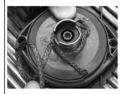
9.6 Remove the center screw and components.
