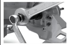
20.33 Install the (2) crankcase guide pins.
