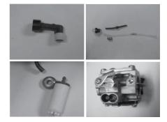
24.3 Remove and inspect the fuel filter.
