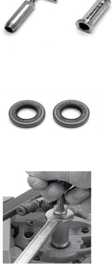
Turn the T-handle until it presses against the shaft and pulls the seal from the crankcase.
