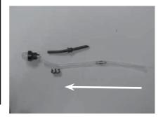
25. This section covers testing the crankcase for leaks. A crankcase leak can cause the engine to run too lean, causing engine damage, or not run at all.
