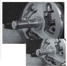
Install the exhaust seal flange.
