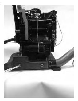
17.2 Remove (2) screws from lower front handle (P/N 544009).
