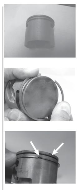
Note ring orientation. \*If rings are installed upside down or incorrectly, ring will not seat properly and piston damage will occur.
