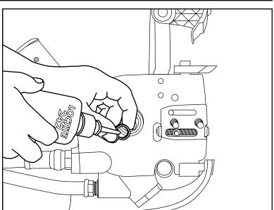
N Make sure it is applied around the entire bore of the seal ring, then slide both parts onto the motor shaft.
