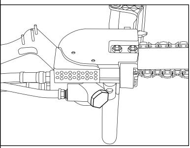
G If the spring washer (14) and spring (15) were removed from the ON/OFF valve, reinstall them. Lubricate the ON/ OFF valve with hydraulic fluid and install it into the valve handle. Secure it in place with the roll pin (18).
