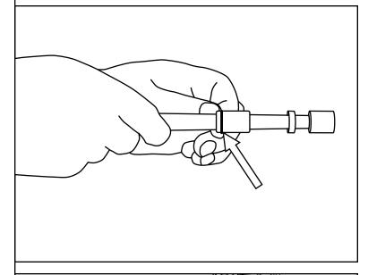
C Apply grease and install new o-ring(31) into the spool bore of the handle.
