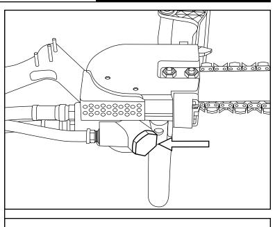
A Unscrew the seal cap (41) and remove it, the o-ring (40), the spring (39), and the steel ball (38).
