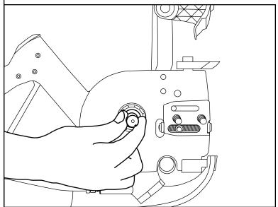
I Turn the motor shaft manually to check for free rotation.
