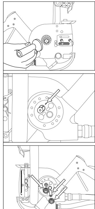
F Slide the drive gear (11) over the needle roller and shaft. Install the idler shaft (6) and gear (7).
