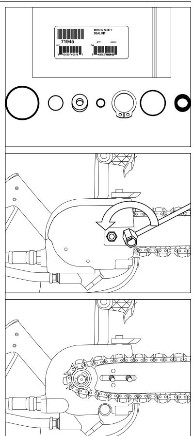
A Remove the 2 nuts (51) and then lift off the side cover (50).
