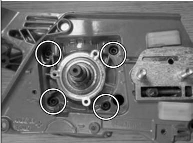
20.22 Install flywheel side crankcase seal – tap with bearing driver and mallet.
