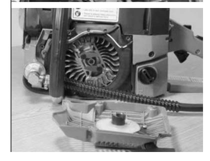
This section covers the removal, inspection, and installation of the flywheel. Removal of the starter and spark plug is required. Refer to sections 6 and 8 if necessary.
