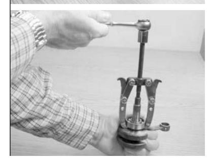
20.9 Remove the bearing, seal, and bushing from the clutch side of crankshaft.
