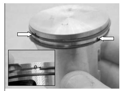
13.15 Install one wrist pin retaining clip.
