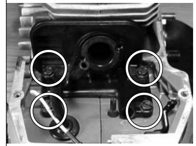
13.2 Remove pulse tube and protective spring from cylinder base.
