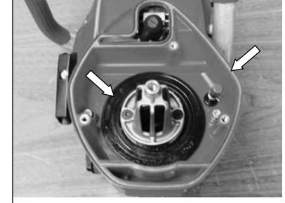
5.6 Secure air filter mount screws.
