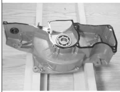
20.19 Place crankcase halves together and align crankcase pins.
