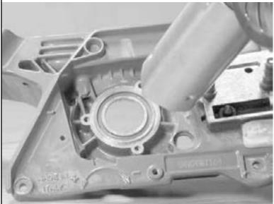
20.12 Install bearing into crankcase halves.
