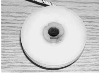
8.11 Install starter rope and tie knot.
