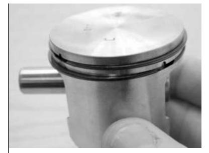
13.18 Align piston in correct orientation.
