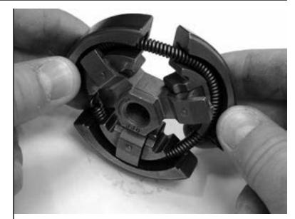
7.8 Finish installation of clutch shoe as shown.
