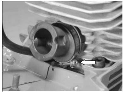
13.5 Remove cylinder screws (4) and wave washers.
