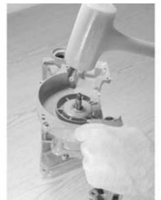
20.5 Remove the flywheel side crankcase seal with 1/2" (13 mm) socket.
