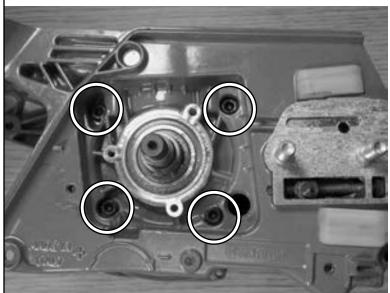
20.3 Heat the flywheel side crankcase with heat gun for 5 minutes, approximately 150° F (65.5° C).
