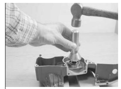
20.15 Install crankshaft into clutch side of case.
