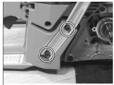
18.2 Remove front handle screws on bottom.
