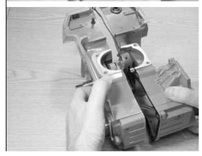
19.20 Assemble crankcase halves – tap with bearing driver and mallet.
