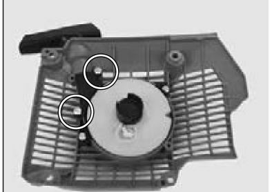
B Line rope up with notch on pulley.
