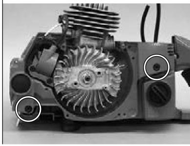
18.3 Separate crankcase and fuel tank.
