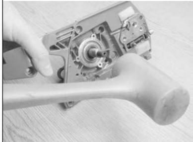
19.8 Remove the bearing from the flywheel side of crankshaft.
