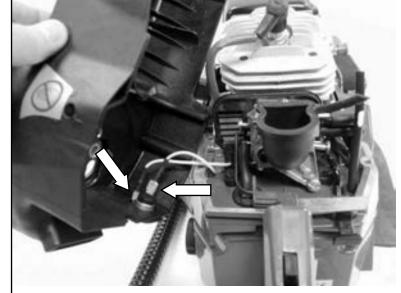
10.12 Make sure carburetor screw boot is in place.
