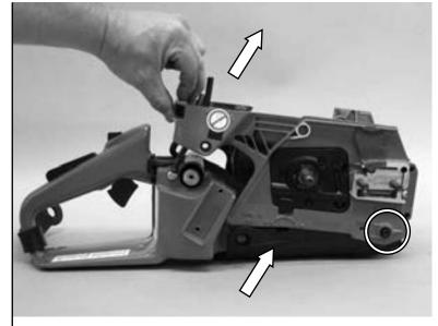
18.4 Remove vibration isolators (4) from fuel tank if necessary.
