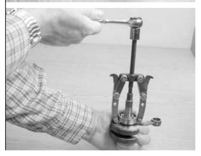
19.9 Remove the bearing, seal, and bushing from the clutch side of crankshaft.
