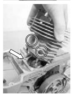
13.7 Remove wrist pin retaining clips (2).
