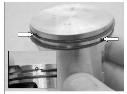
13.15 Install one (1) wrist pin retaining clip.
