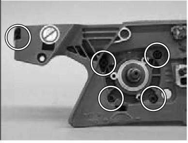
19.3 Heat the flywheel side crankcase with heat gun for 5 minutes, approximately 150° F (65.5° C).
