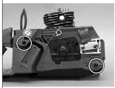
18.2 Remove vibration isolator screws (2) and wave washers on flywheel side of saw.
