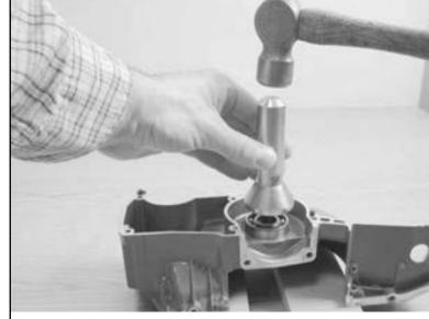
19.15 Install crankshaft into clutch side of case.
