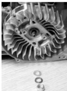
16.3 Screw on flywheel removal tool finger tight. Unscrew tool 1 ½ turns leaving approximately 1/8 inch (4 mm) space between tool and flywheel.
