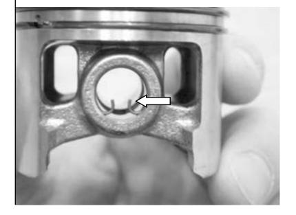
13.17 Lube and partially install wrist pin.
