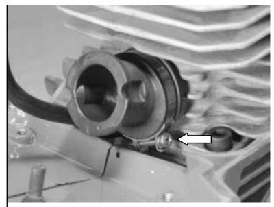
13.5 Remove cylinder screws (4) and wave washers (2 on front and 2 on back)
