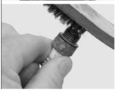
6.5 Gap if necessary to 0.02" (0.5 mm).
