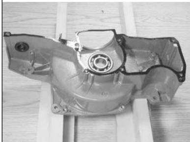
19.19 Place crankcase halves together and align crankcase pins.
