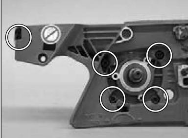
19.22 Install flywheel side crankcase seal – tap with bearing driver and mallet.
