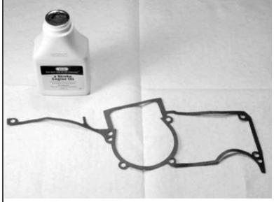
20.18 Align crankcase gasket on flywheel side crankcase pins.
