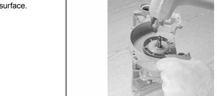
20.5 Remove the flywheel side of crankcase seal.
