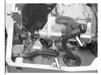
12.3 Remove carburetor attachment screws.
