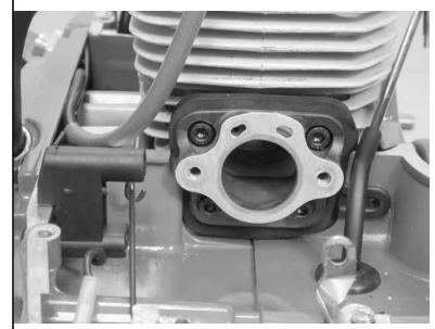
13.2 Remove cylinder screws (4) and wave washers.
