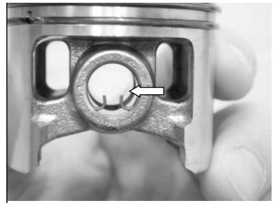
13.14 Lubricate wrist pin and partially install in piston.
