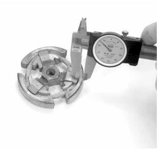
7.7 Inspect spring for cracks.
