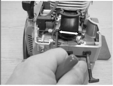
12.4 Remove intake manifold.
