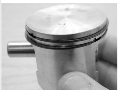
13.15 Align piston in correct orientation.
