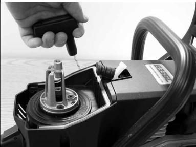
7.3 Remove clutch shield with small screwdriver.
