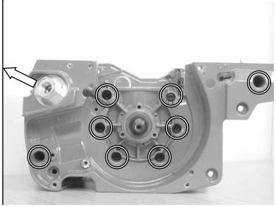
20.3 Heat the flywheel side of crankcase with heat gun to 150° F (65.5° C).
