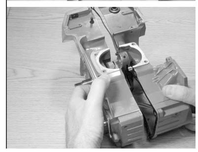
20.20 Assemble crankcase halves; tap with bearing driver and mallet.
