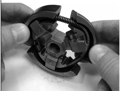
7.9 Finish installation of clutch shoe as shown.
