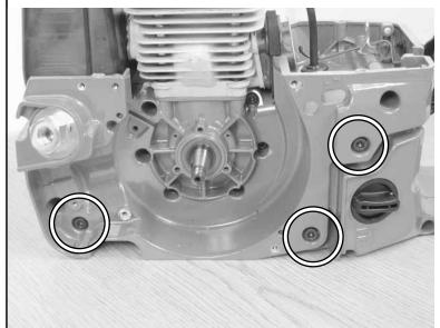
19.3 Separate crankcase and fuel tank.
