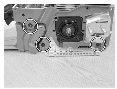
19.2 Remove vibration isolator screws and wave washers on flywheel side of saw.
