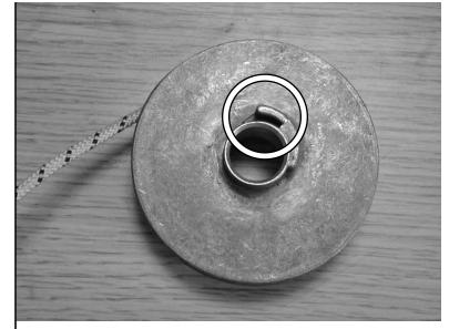
8.11 Install starter rope and tie knot.
