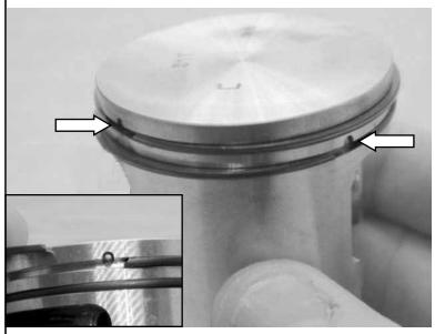
13.12 Install one wrist pin retaining clip.
