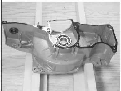
20.19 Place crankcase halves together and align crankcase pins.
