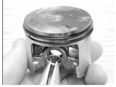
13.13 Make sure wrist pin retaining clip is in the proper orientation.
