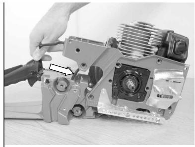
19.4 Remove vibration isolators from fuel tank (6) if necessary.
