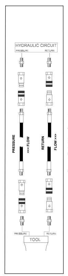
Figure 1. Typical Hose Connections
