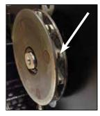
SPROCKET WEAR: Inspect sprocket after each usage. Replace when grooves in the drive teeth are worn more than half way through (approximately every 2-3 chains) and resembles the photo above.
