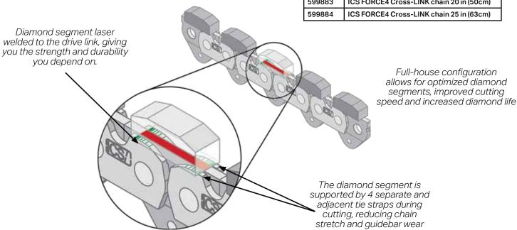
Drive Links, Tie Straps and Segments work in concert to prevent reverse articulation and increase stability in the cut, providing a smoother cutting experience with less operator effort
