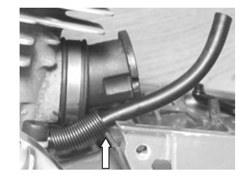
Remove rear manifold clamp.
