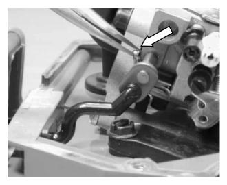
Remove carburetor support screw (1) with #4 Torx or straight blade screwdriver.
