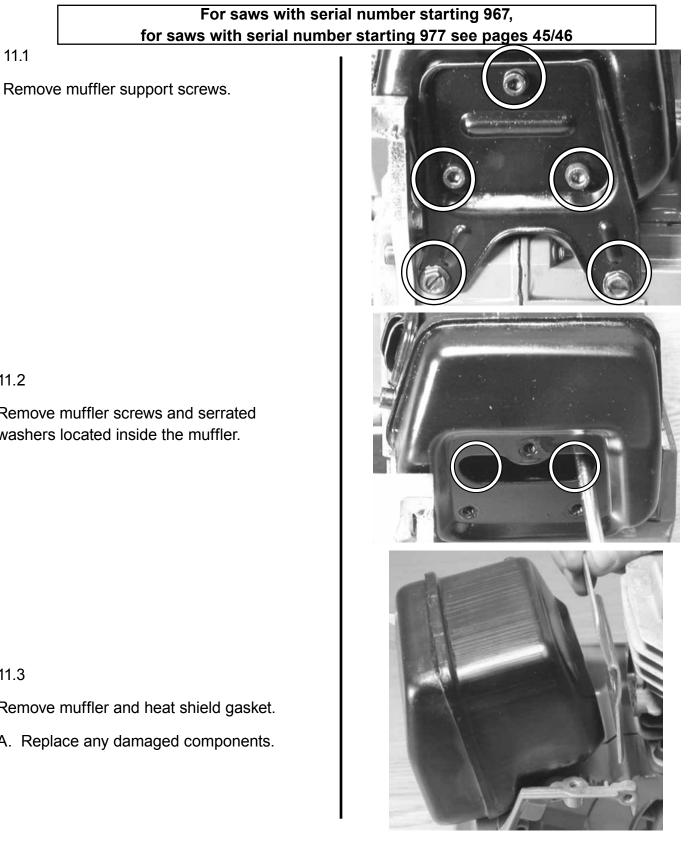
Remove muffler screws and serrated washers located inside the muffler.
