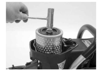
11. This section covers the disassembly, inspection, and assembly of the muffler. Removal of the WallWalker® and cylinder cover is necessary. Refer to sections 7 and 10 if necessary.
