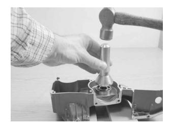
Install crankshaft into clutch side of case.
