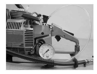
The fuel tank breather stabilizes the pressure in the fuel tank preventing both excessive pressure, which could flood the engine, and negative pressure, which could starve the engine of fuel.
