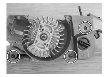
Separate crankcase and fuel tank.
