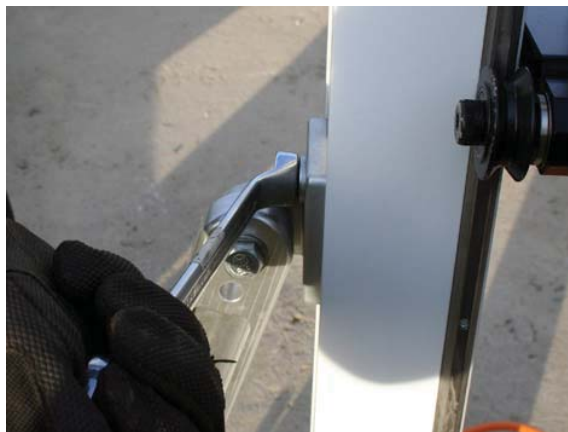
e. When the track is in the right position, tighten the bolt properly.
