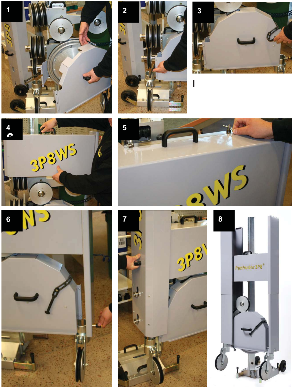
Fitting of guard on Pentruder 3P8 wire saw.
