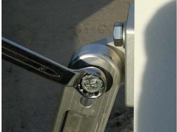
a. Loosen the upper bolt on the back support.
