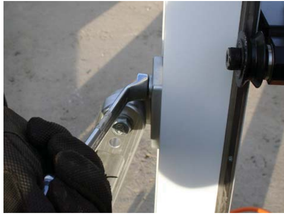
e. When the track is in the right position, tighten the bolt properly.
