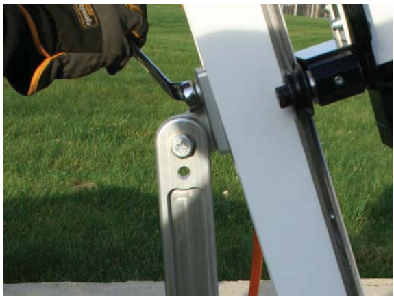
c. Loosen the bolt on the upper brace and tilt the track to the wanted positioned backwards or forwards.
