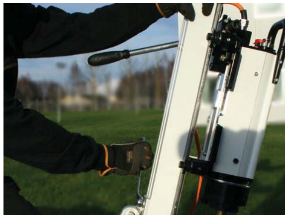
d. Tighten the bolt on the lower brace and the upper and lower bolt on the back support.
