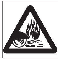
Fire risk due to sparks
