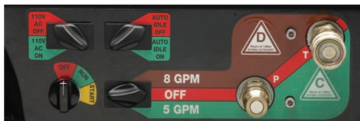
Figure 1. Panel Control Valve
